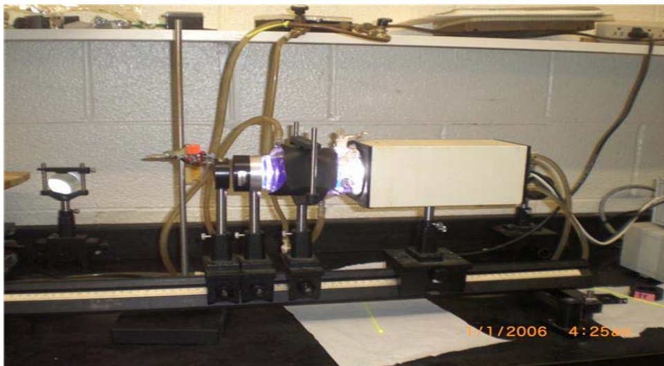
Figure 5. Illumination set-up consisting of 150 W xenon lamp, copper sulfate solution, two glass filters to give 440 nm light and the sample which contains Mn (III) Por + .
